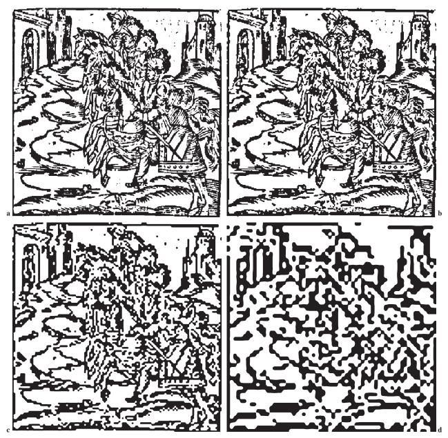
1 Four resolutions of same picture illustrating effect of non-linear median filter ((a) is original image with all detail; (d) keeps only the image main features): (a) binarized original image at resolution 0 (512 × 512 pixels); (b) resolution 1 (256 × 256 pixels); (c) resolution 2 (128 × 128 pixels); (d): resolution 2 (64 × 64 pixels)
